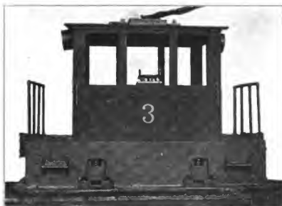
Fig. 4672. Baldwin-Westinghouse Electric Locomotive for the Pennsylvania Steel Co. Weight, 28,000 lbs.; Diameter of Drivers, 30 in.; Wheel Base, 5 ft. 6 in.; Drawbar Pull, 5,600 lbs.; No. of Motors, 2.
